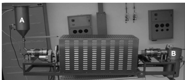
Figure 1 View of the rotary tube furnace used for large-scale synthesis of CVD. A: Catalyst stock continuously driven inside the 3 inch quartz tube. Raw materials (CNTs + Catalyst) are collected in B
